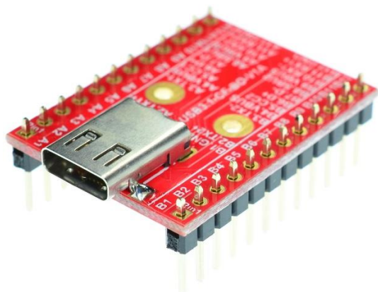
Figure 3: USB3.1-CF-BO-V1A with headers
