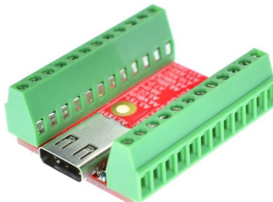
Figure 4: USB3.1-CF-BO-V1A with terminal blocks
